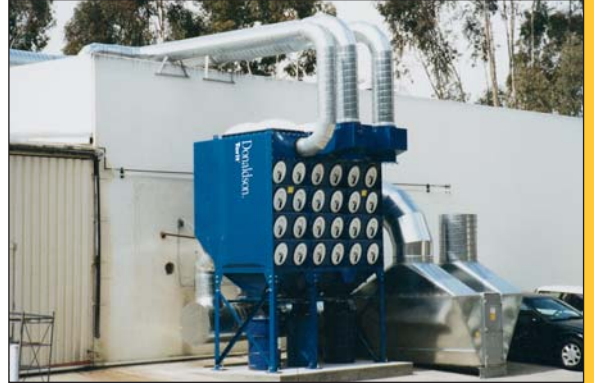
DFO 4-48 on metal grinding
