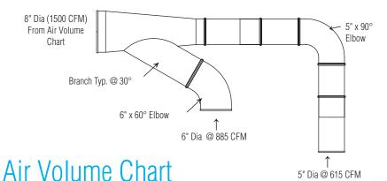
The 5" pipe carries 615 CFM at 4500 FPM, (See chart). The 6" pipe will need 885 CFM at the same velocity (See chart). Added together you have a total of (615 + 885) 1500 CFM coming together.
