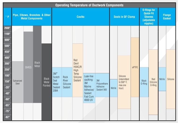
This information is intended as a general recommendation. Each component in a ductwork system should be analyzed for temperature vulnerabilities (example: Rubber seals in blast gates have a lower temperature rating than the metal housing.) See individual product pages for notes regarding components with additional temperature limitations.
