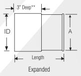
Adapters can only be expanded up to .3" above the nominal diameter size (A dimension). Expansions larger than .3" must be ordered as a reducer.
