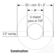
Seam: Spot welded and caulked.
