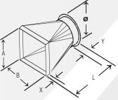
**Hood Design Basis:** 150 fpm capture velocity 2 ft. distance from source
