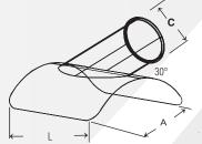
Saddle length and width = 3" all directions from Branch Tube C.
