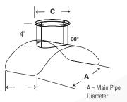
Saddle length and width = 2" all directions from Branch Tube C.
